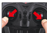
Chart 1: Enter into compass calibration, aircraft indicator will blink red and blue alternately
