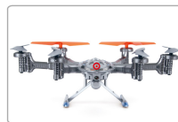
Chart 4: The red indicator light solid means calibration is successfully, and then put the aircraft at horizontal place.
