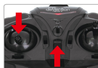
Chart 2: Pull down throttle control sticker to the lowest position and then turn on the radio.
