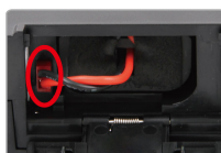
Chart 1: connect the battery of the radio
